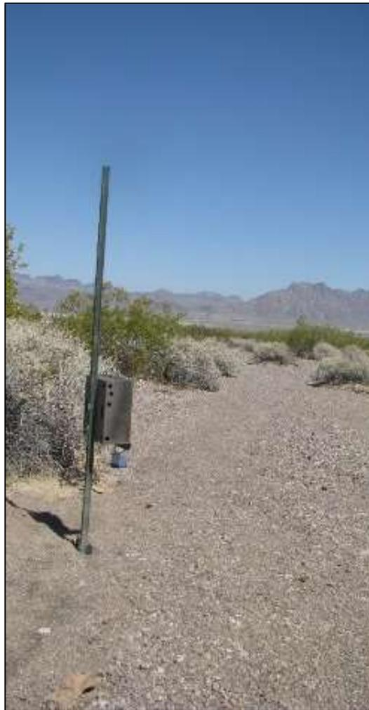
Figure 4. Example of a randomly placed grid camera in the BCCE during 2018. The lock box was necessary in this highly visited area to prevent theft. The T-post is driven into the ground with a sledge and the lockbox was attached with U-bolts.
